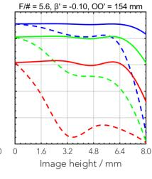
— 20 LP/mm, radial— 40 LP/mm, radial— 80 LP/mm, radial--- 20 LP/mm, tangential--- 40 LP/mm, tangential--- 80 LP/mm, tangential
