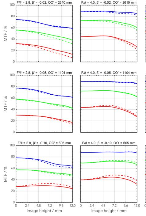
— 80 LP/mm, radial – 20 LP/mm, radial - 40 LP/mm, radial --- 20 LP/mm, tangential --- 40 LP/mm, tangential --- 80 LP/mm, tangential
