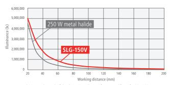
\* Measured at each of the above given distance from an end face of a Ø8, 1100-mm long straight light guide at 100% illuminance (Not guaranteed)
