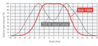
\* Measured at a 600-mm distance from an end face of a Ø8, 1100-mm long straight light guide at 100% illuminance (Not guaranteed)
