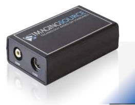
Despite the fast growing world of digital cameras, there is still an enormous number of analog video sources. Using a Video-to-USB converter, such as the DFG/USB2pro and the DFG/USB2aud, analog video sources become usable in a digital environment.
