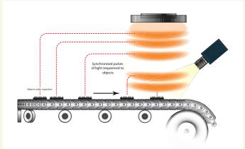
Strobing or pulsing of the lighting can freeze fast moving action as shown below
